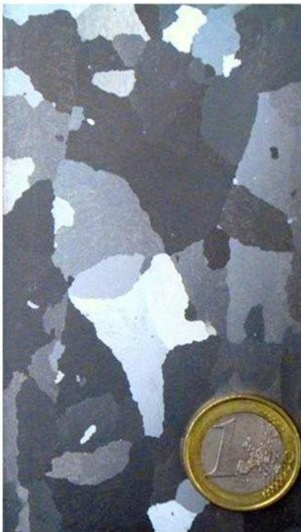
Goss texture in Silicon steel (electrical steel)
